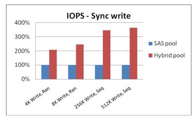
Figure 5 Hybrid pool and SAS pool with synchronous write
