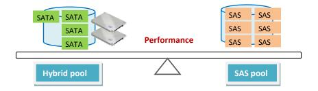
By using read-optimized SSD and write-optimized SSD, the overall performance of hybrid SATA storage pool can be close to or better than that of a SAS storage pool in two distinct ways - synchronous write applications and deduplication. The extra benefits are lower costs, more capacity, and lower power consumption if compared with full SAS solution.
