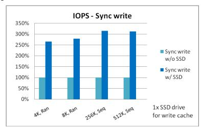
Figure 4 Compare write performance using 1x SSD drive as write cache
