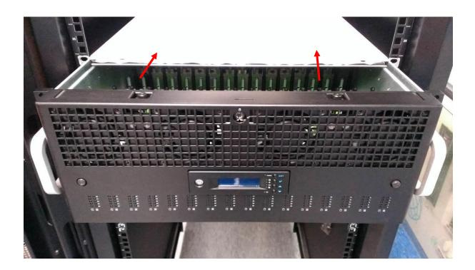
C. Loosen the two thumbscrews from the Master Expander Module.
