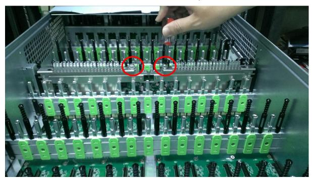
D. Carefully remove the Master Expander Module.
