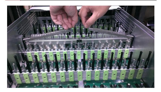
E. Check the Master Expander Module's pin connectors. Make sure there are no bent pins.
